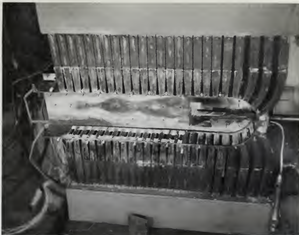
Figure 8 - Combustion Chamber Showing Lower Injection Orifices as Modified.
